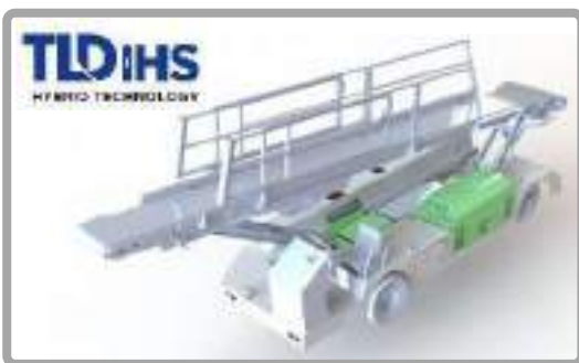
3D drawing of the iHS drive unit
